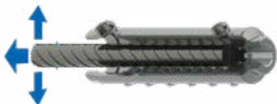
Allows connection of continuation bars that are not perfectly aligned: Misalignments of up to 12mm for small bars (Ø12-Ø20), up to 20 mm for medium bars (Ø25) and up to 25 mm for large bars (Ø28-Ø40) can be accommodated.
