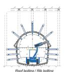
Dextra GEOTEC Steel Self-Drilling Rock-bolt is primarily designed for tunnelling and mining, for roof and wall bolting in various ground conditions, but can also be used as a ground anchor, both active or passive.
